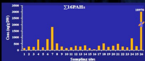
Figure 3. Concentration of Σ16PAHs in sediment samples collected from different locations between Ko Sichang and Siracha in February 2011.
