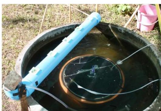
Figure 1. Experimental setup showing concrete tank, two-staged filter (at center) and hydroponic pipe.
