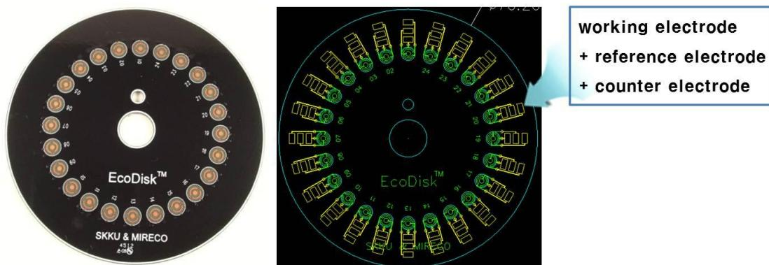
Figure 1. Photograph of the fabricated heavy metal detection lab chip for on-site measurement
