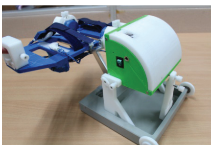
Figure 2. Supporting parts attached to the robot for movements of the elbow flexion-extension (left), for the wrist flexion-extension (middle) and the forearm pronation-supination (right)
