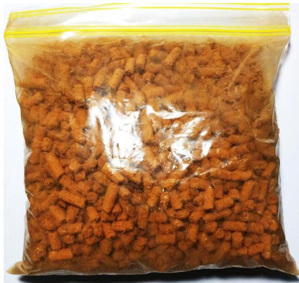
รูป 3.11 Ferric Oxide Desulfurizer (coal based)
