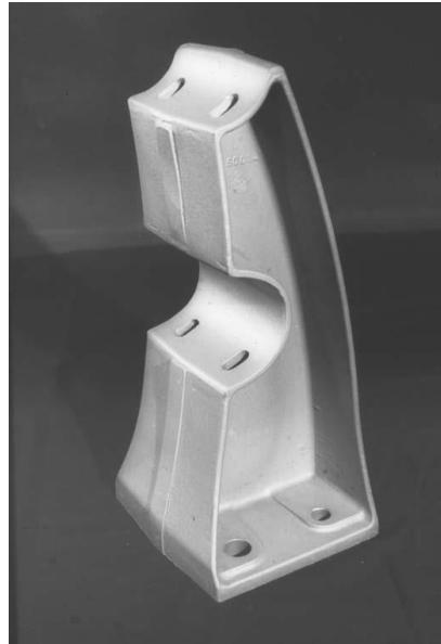
รูปที่ ก.1 Example of one of the many highway railing post designs utilizing aluminium castings that have been developed. The alloy is A444.0- T4 with minimum elongation in permanent mold castings of 20% in front flanges for maximum energy absorption during impact.
