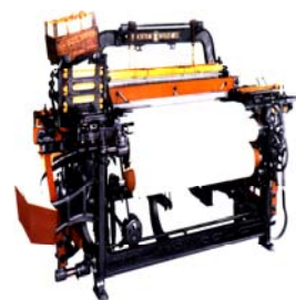
Type-G Toyoda Automatic Loom with Non-stop Shuttle Change Motion
