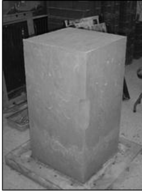
Figure 2.13 Tested specimen decreased by 200 times 0.50x0.50x0.95 m 3 (Tunsakul et al., 2013)
