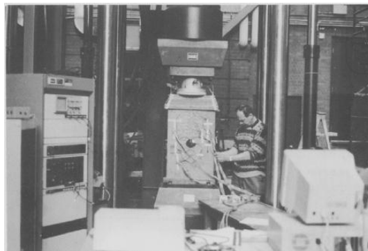
Figure 2.12 Testing of a large granite block ( R = 50 mm) (Dzik and Lajtai, 1996)
