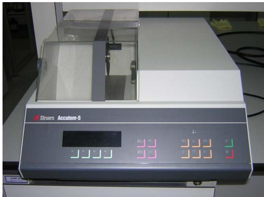
**Fig. 2.2** Cutting machine model ACCUTOM-5 from Struers Co.
