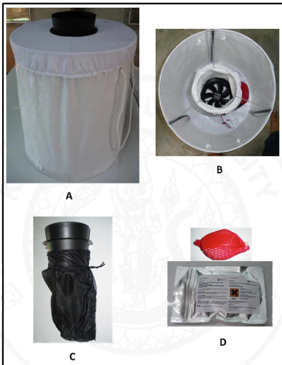
Figure 4 The BG- Sentinel (BGS) TM trap, external view (A), inside view showing fan and lure pouch (B), the black funnel where mosquitoes enter with the catch bag (C) and the accompanying BG-Lure (D).
