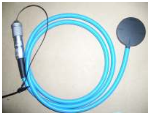
Figure 4.6 The Roos chamber type 34001
