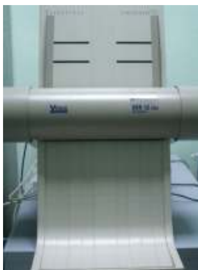
Figure 4.5 The VXR – 12 plus film digitizer
