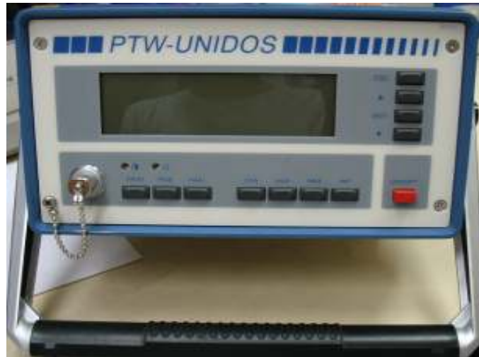
Figure 4.7 The PTW UNIDOS electrometer
