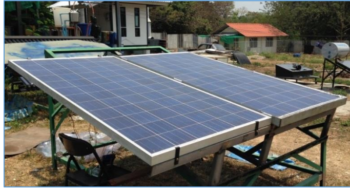
Figure 3.2 Module solar cell PV-R (left) and PV-PCM (right).
