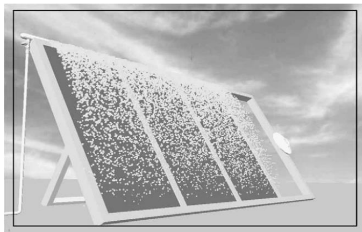
Figure 1.7 Cooling solar cell by water flow [9].
