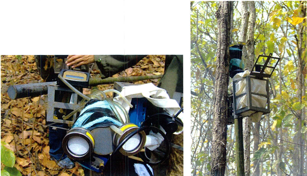
Figure C.6 Field equipment set up in the box at the top of tower height 3 m
