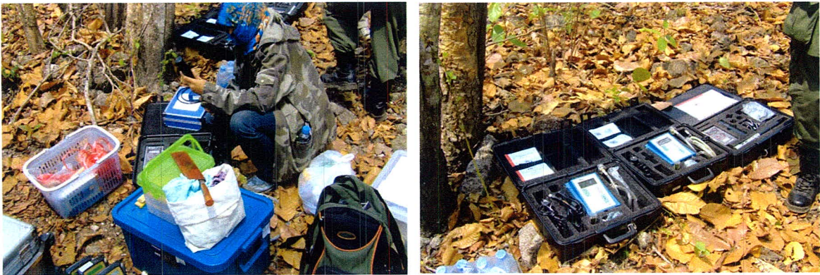
Figure C.5 Field equipment set up for emission pollutant sampling from prescribed fires
