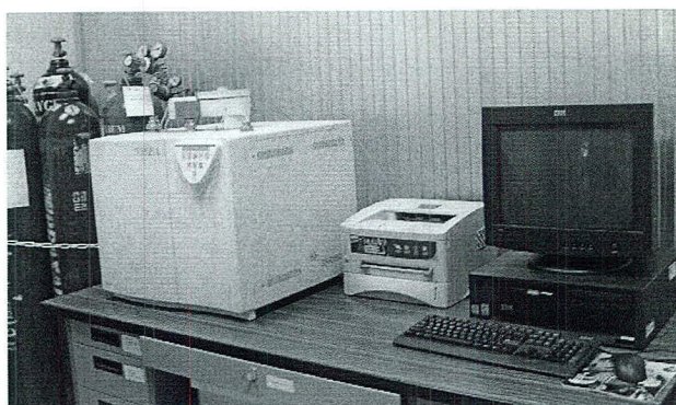
Figure B.5 OEA analyzer FlashEA1112 (Thermo Finnigan, Italy) instrumental configuration used for carbon content analysis in PM emitted from biomass burning.
