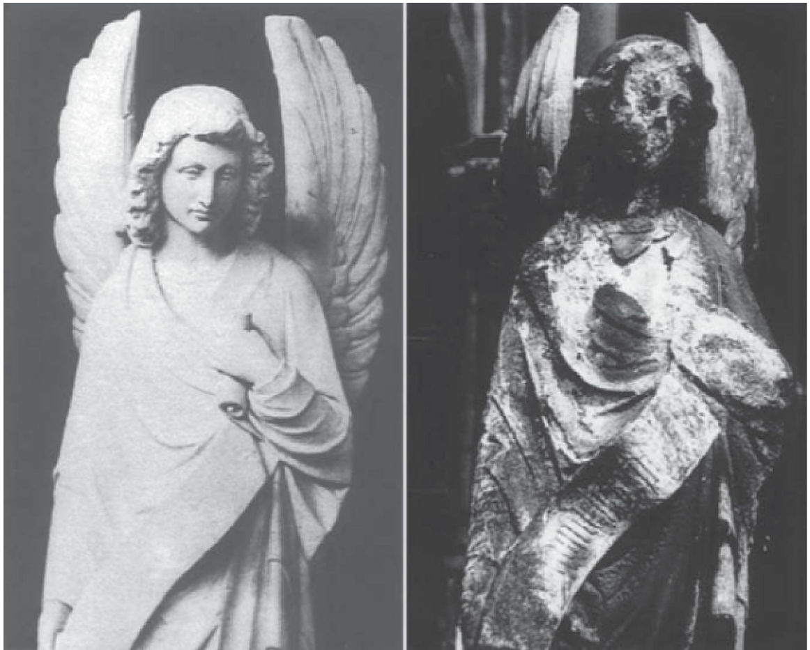
Fig. 43 Effect of pollution caused deterioration on the statue of an angel at the cathedral of Cologne, Germany: (a) picture taken in 1880, (b) the same statue in 1993. From Warscheid and Braams photos (Mitchell and Gu 2010, p. 138)
