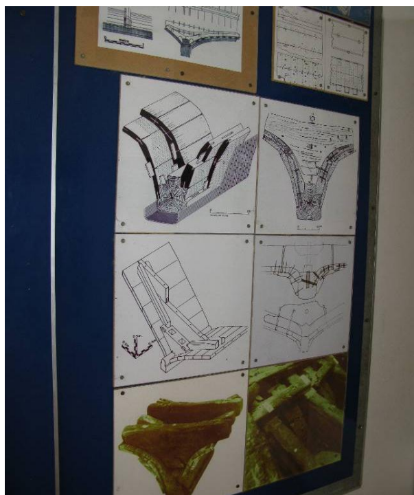
Figure 168 The remains of a keel have the same structure as a European ship. The bottom of the ship was made by following the European pattern or Dutch technology. Photograph by Phungwong, N. on August 22, 2010.
