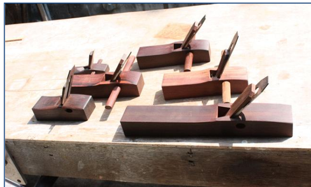
Figure 157 A plane set in Thailand which is similar to Dutch wood working tools. These planes are used to build Thai houses or wooden boats. They come in different sizes for various purposes. Photograph by Phungwong, N. in April 2010.
