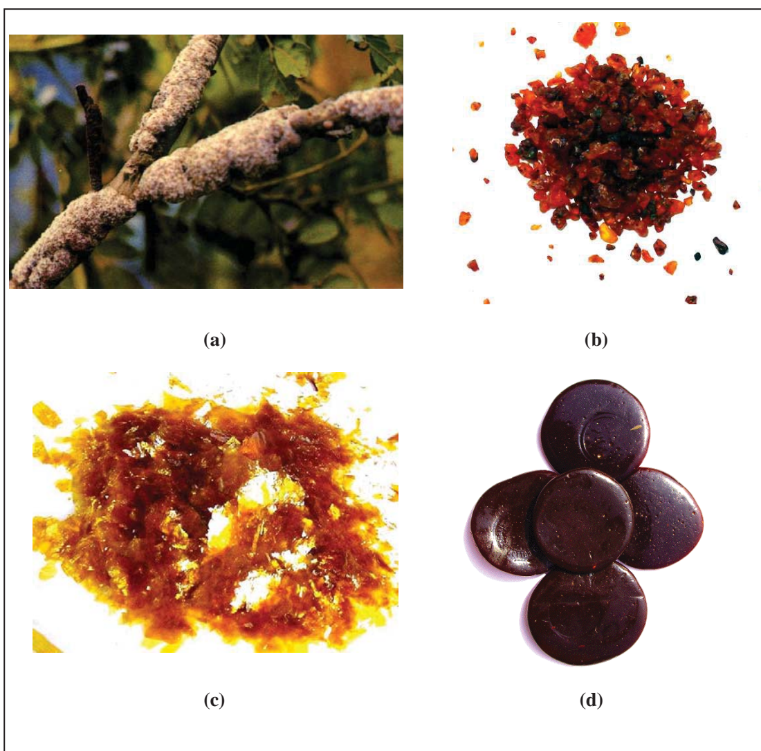
Figure 6 Stick lac (a), seed lac (b), shellac (c), and button lac (d)
