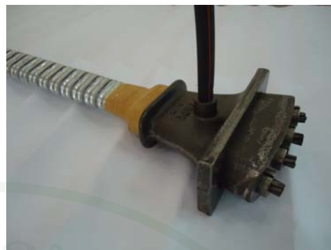
(e) Tendon (fabrication of strands and hard-ware)
