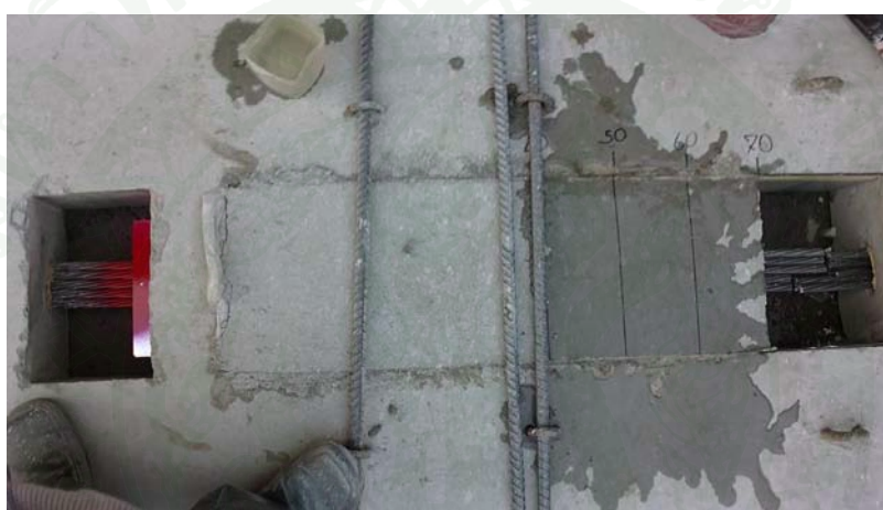
(a ) Checking the slip in slip checking point at left end after transfer the anchorage force and refer to the marking reference point in step 3.5 as shown in (b) and (c).
