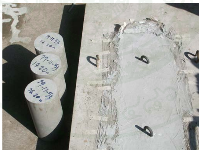
(b) Compressive strength test to refer to strength of concrete in bonded length box.
