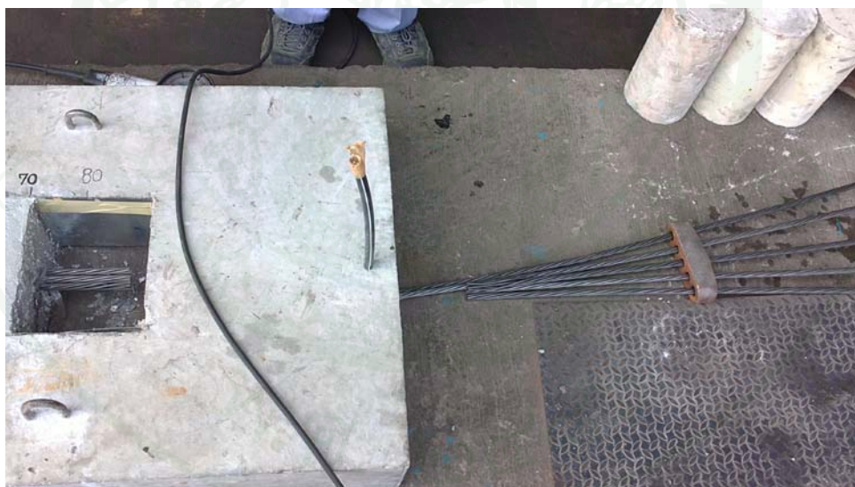
(b) Force at anchorage reduced to zero.
