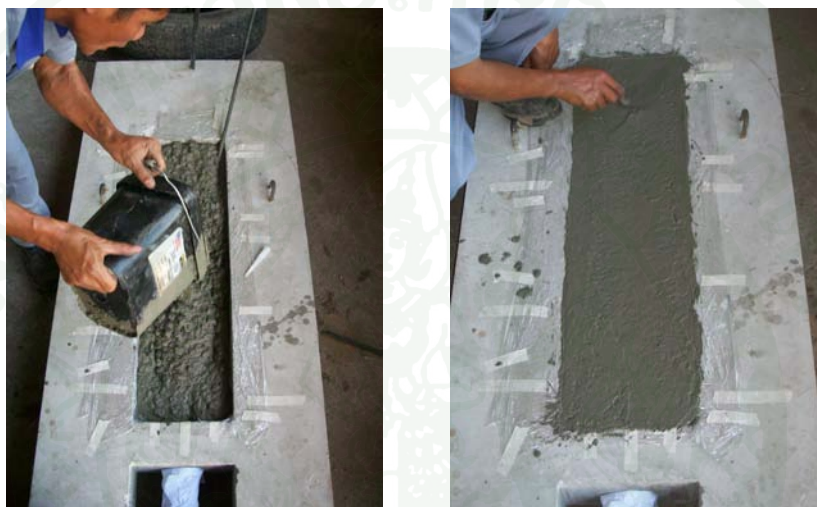
Figure 28 Casting of concrete in to the bonded length box.
