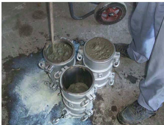
(a) Sampling concrete for compressive strength test
