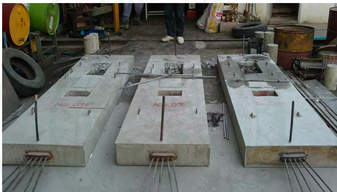
Figure 38 The 3 specimens of the test block of multiple 5-strand tendons after test.
