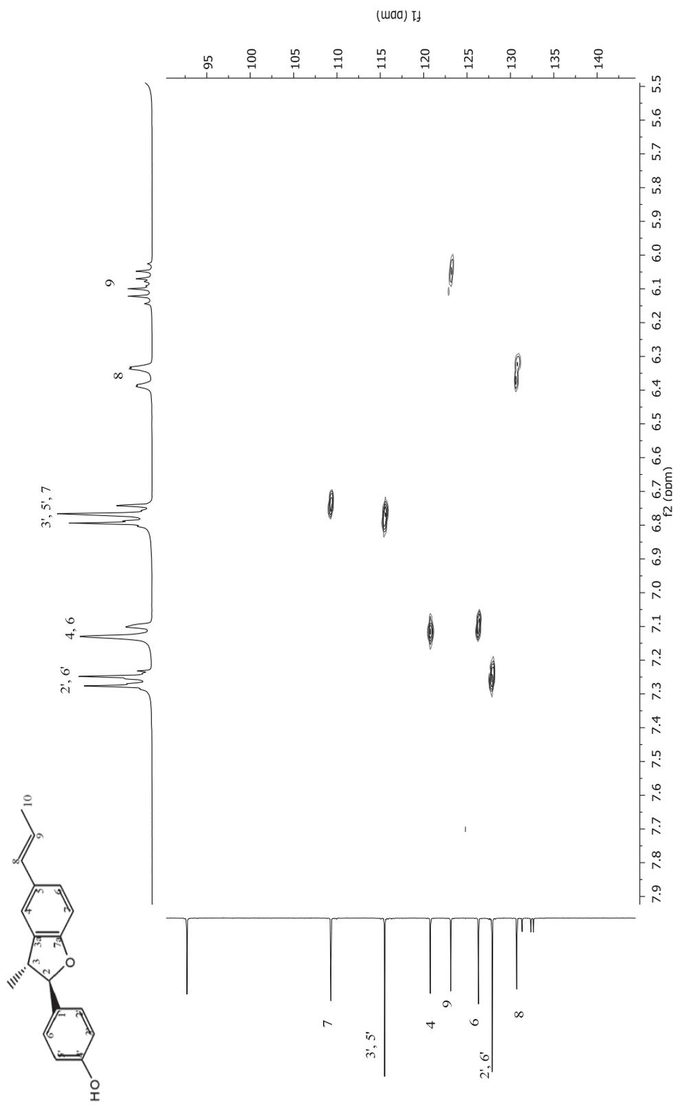
**Figure 115** (Continued) HMOC Spectrum of compound MHL-3 (in CDCl<sub>3</sub>)
