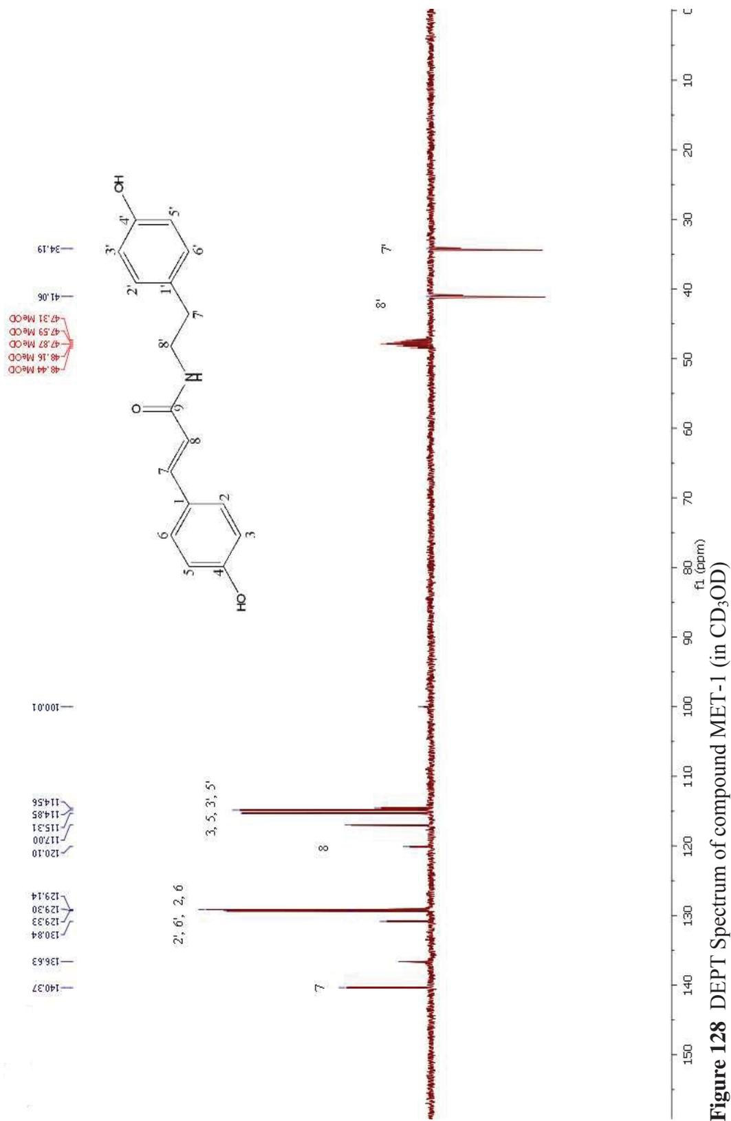
**Figure 128** DEPT Spectrum of compound MET-1 (in CD<sub>3</sub>OD)
