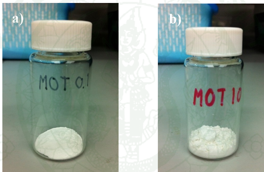
Figure 39 Images of the M-S-H synthesized using Mg/Si ratio at a) 0.1 and b) 1.0
