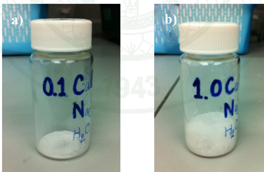
Figure 24 Images of the C-S-H samples synthesized using \text{Na}_2\text{SiO}_3 at Ca/Si ratio a) 0.1 and b) 1.0
