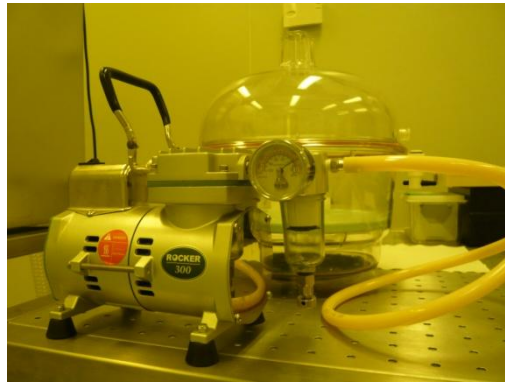
FigureB.3 Evacuated the air in PDMS
