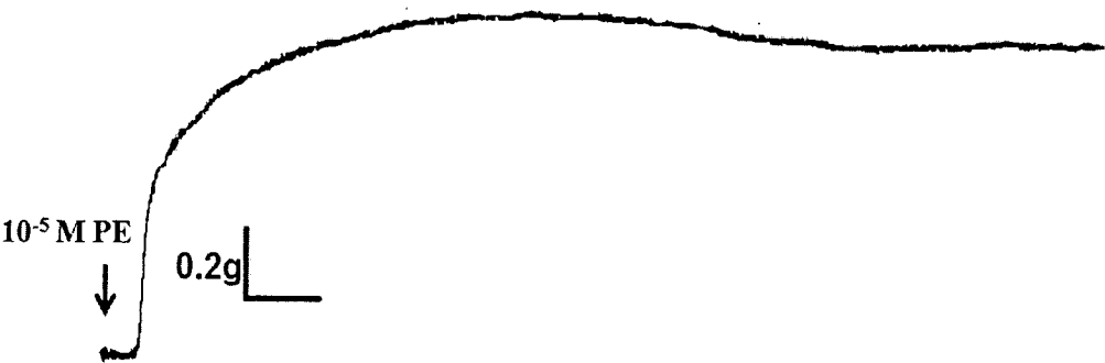
Figure 25 Typical trace of contraction induced by 10^{-5} M PE after 45 min on pulmonary artery
