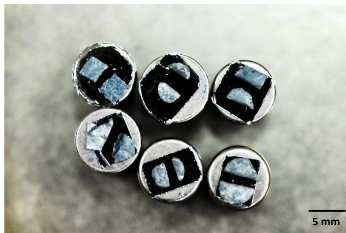
Figure 3.17 The dried samples were coated with gold for SEM observation and EDS analysis.
