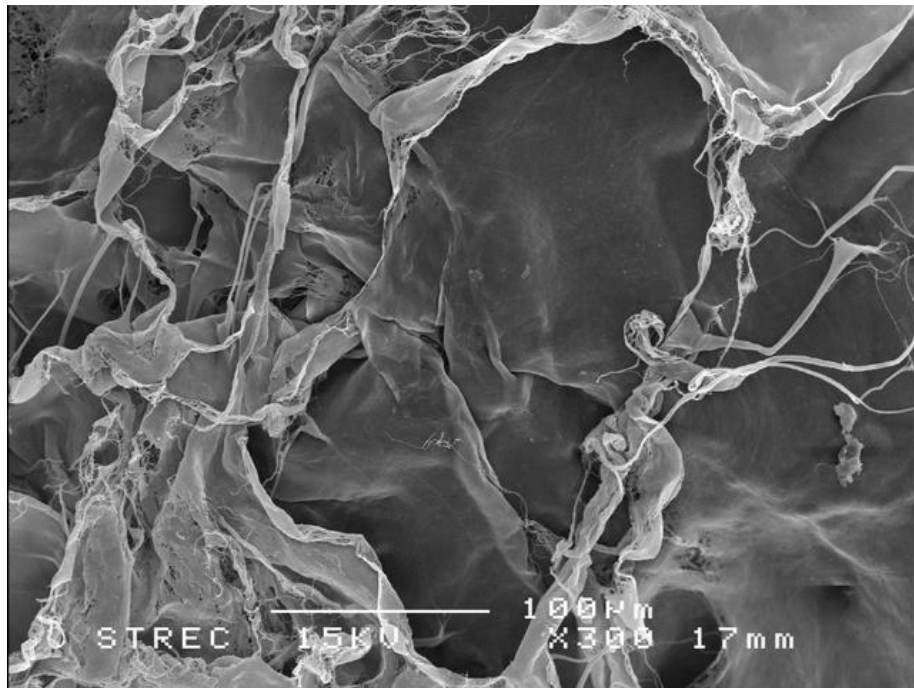
Figure 4.17 SEM observation of type I collagen scaffold without cells.
