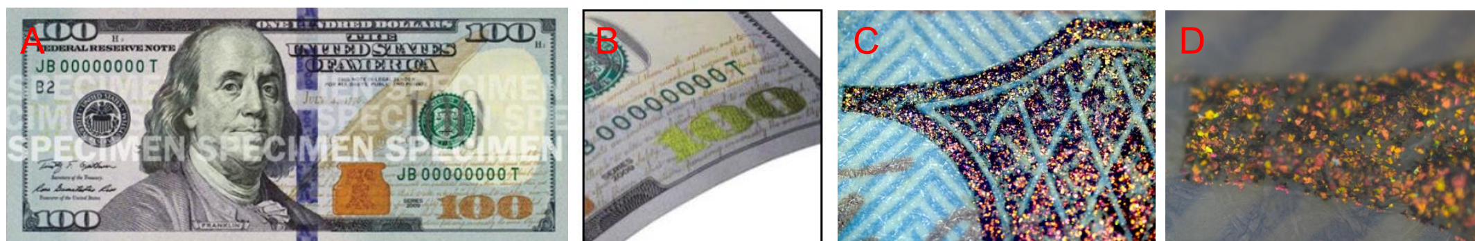
Figure 1. Color-shift printing on $100 bank note. When the bank note was tile, the color of number 100 changes from copper red to green (A-B). Optical microscope (OM) images observed with 5X (C) and 20X (D) objectives of mica pearlescent pigment.
