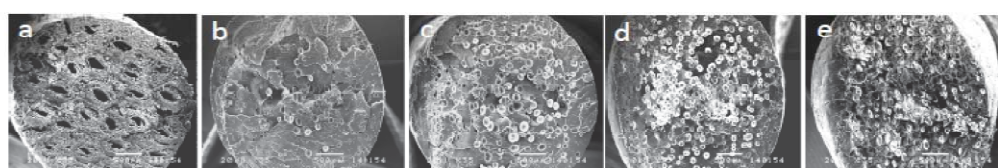
Fig.5. Cross-sectional morphology of natural rattan (a), and foamed synthetic rattan with CFA of 0.5 (b), 1.0 (c), 1.5 (d), and 2.0 (e) phr.
