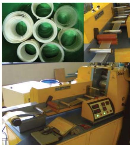
**Figure 63.** Extrusion sheet process and PLA,  $CaCO_3$ -PLA nanocomposite and plasticized  $[SiO_2-CaCO_3]$ -PLA nanocomposite sheets.
