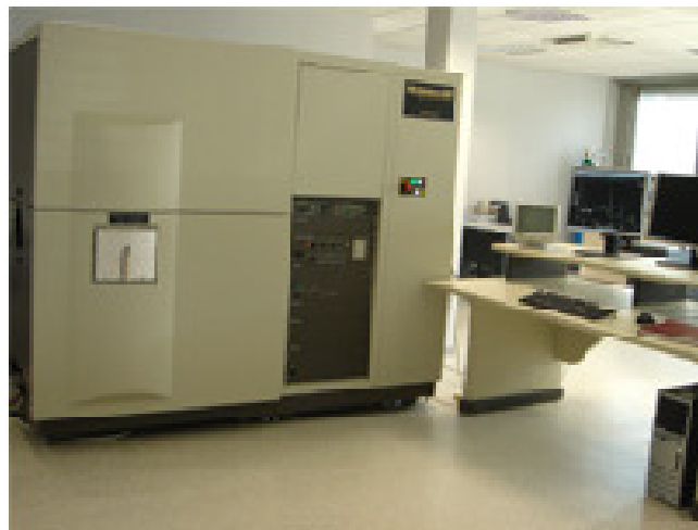
Figure 3.5 Image of PHI Quantera II XPS Scanning Microprobe system
