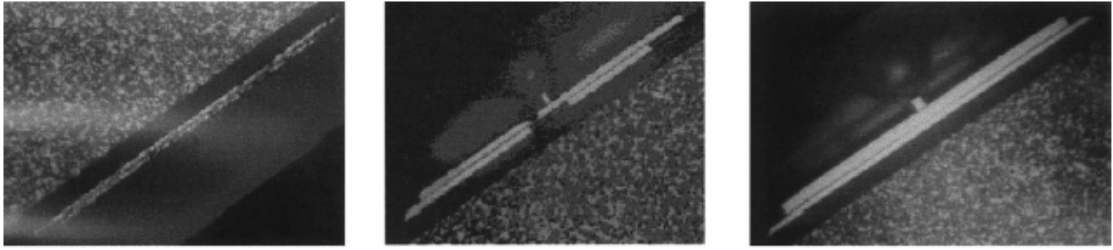
Figure 2.23 Acid etch corrosion test results for sliders with: (a) no overcoat; (b) ion beam CVD DLC, 5 nm; and (c) FCA coated ta-C, 5 nm.
