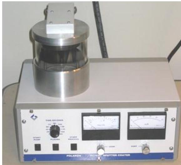
**Figure 2.40** Sputtering deposition
