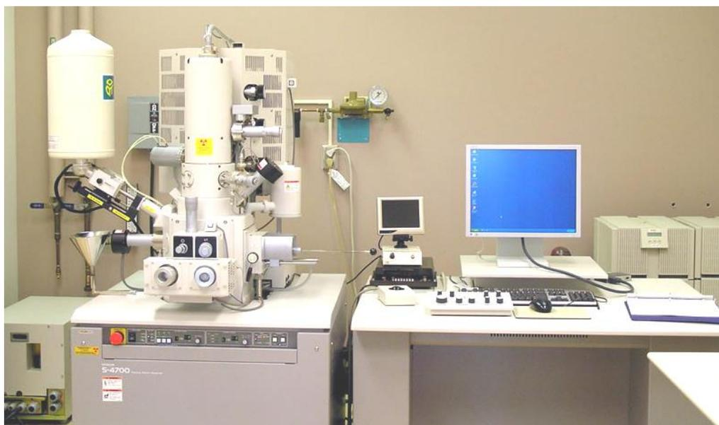
**Figure 2.21** Scanning electron microscopy [45]
