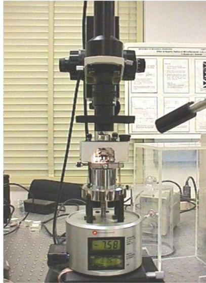
**Figure 2.25** Atomic Force Microscope
