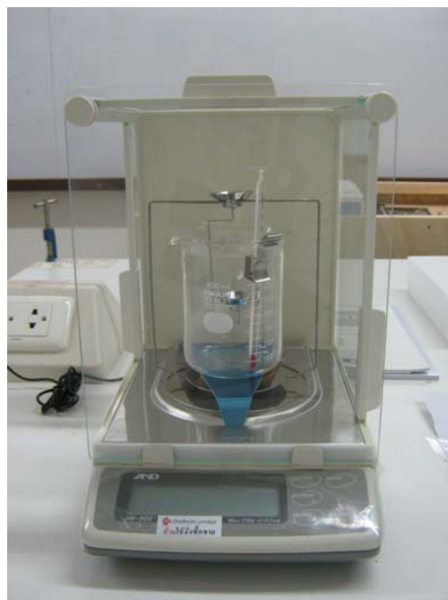
Figure 3.7 The sensitive microbalance for density determination.
