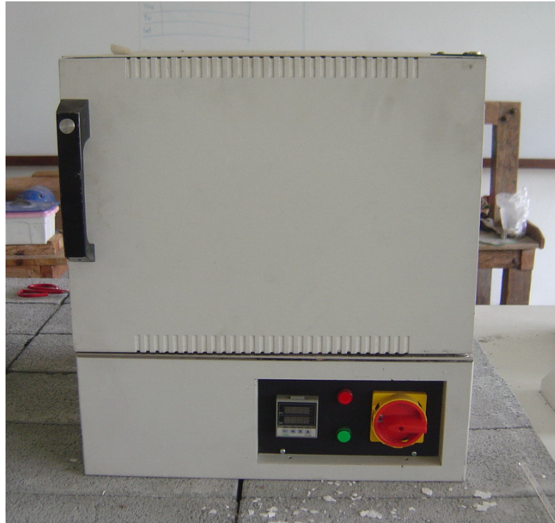
Figure 3.6 High temperature electrical furnace for glass annealed.
