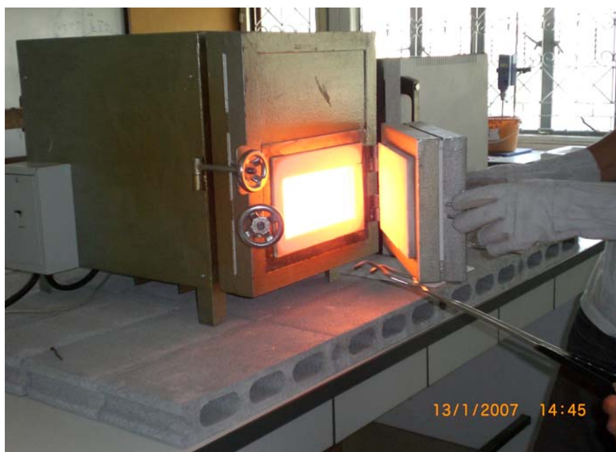
Figure 3.5 High temperature electrical furnaces for glass melting.
