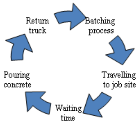
Figure 3.1: Ready mixed concrete delivery process
