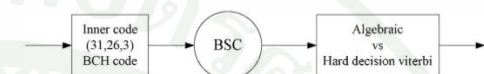
Figure 2. System setup for hard decision decoding using algebraic decoding in comparison with VA
