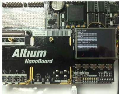
Figure 8. An example of the concatenated encoding result shown in the TFT-LCD display on the Nanoboard 3000 board.
