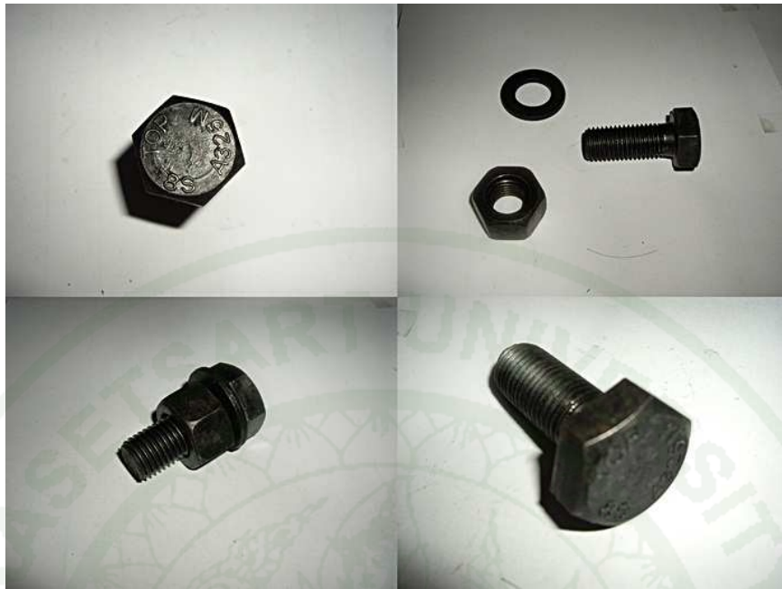
Figure 7 ASTM A325 bolts, diameter 16.0 mm
