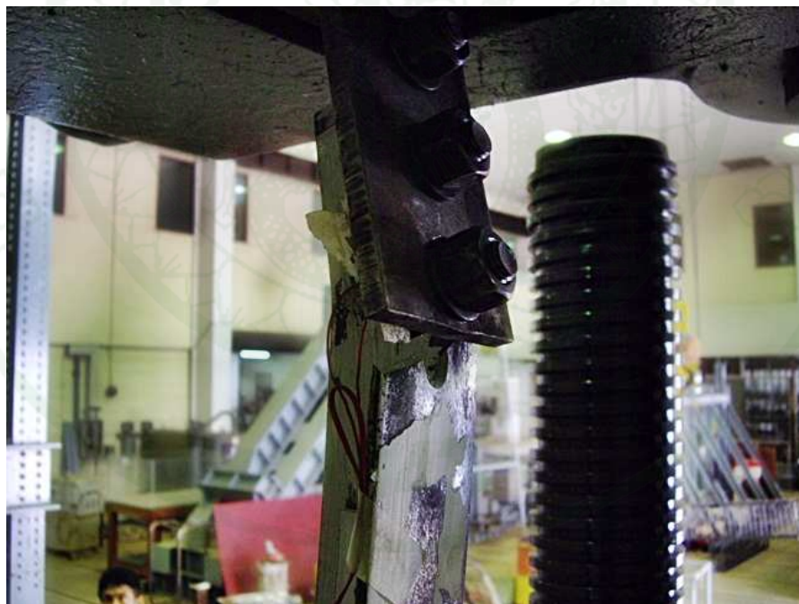
(c) Bent gusset plate during the test
