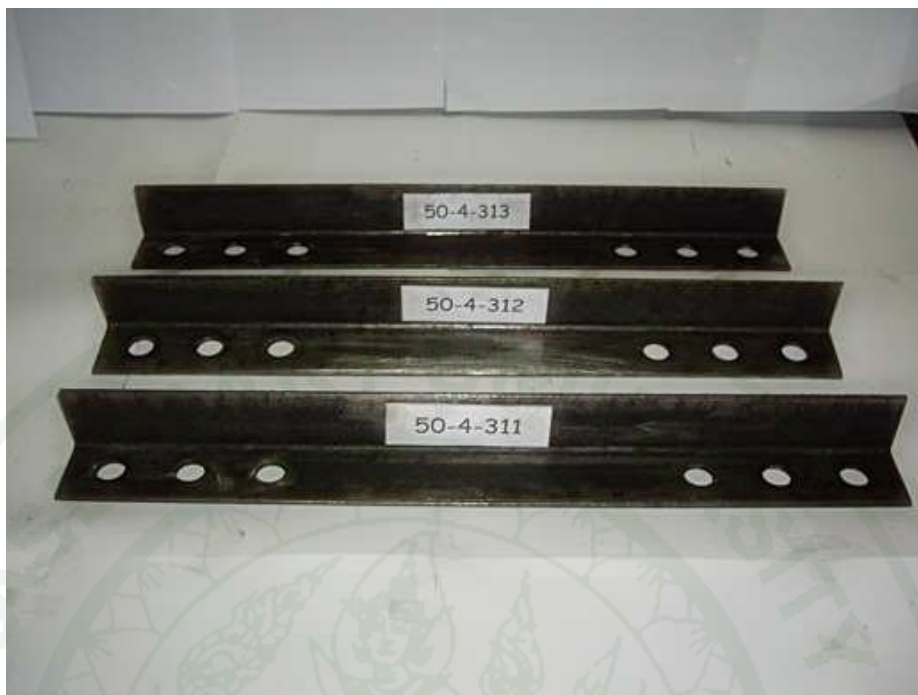
Figure 16 Angle section 50x50x4THK., 500mm length
