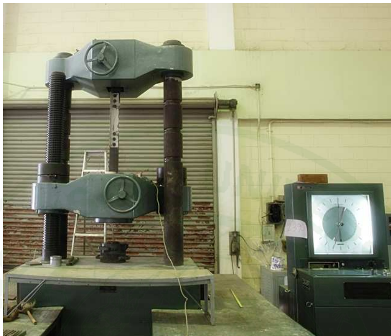
Figure 9 Universal Testing Machine (UTM) with monitor, Capacity 2000 kN.
