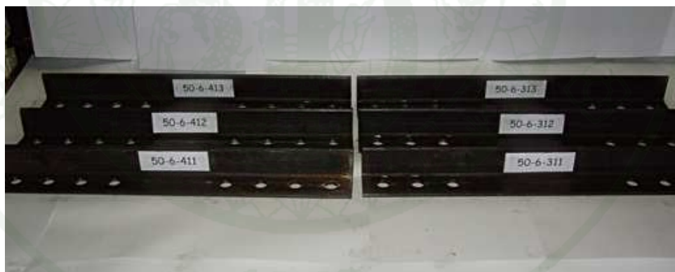
Figure 17 Angle section 50x50x6THK., 500mm length.
