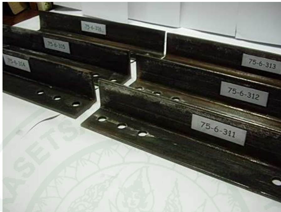
Figure 18 Angle section 75x75x6THK., 500mm length.
