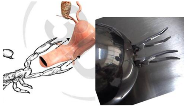
Fig.2. The right and left chelicerae of the scorpion- like robot were able to grip and manipulate the ligaments and vessels at parametrium. (black arrow)
