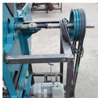
Figure 2. Power measuring device
