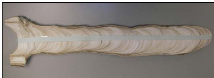
Figure 3-8 Graph paper lay on top of the cut surface of stalagmite NJ1 for drilling
