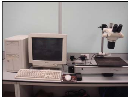
Figure 3-12 The equipment for tree ring width measurements (TSAP version 3.2)
