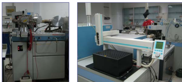
Figure 3-9 MAT-253 mass spectrometer linked to a Gas Bench-II (Thermo-Finnigan) machine
