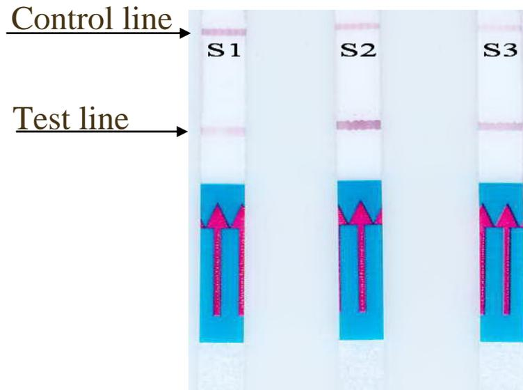
**Figure 16.** Photograph of results from FITC probe optimization for detection of HPV amplicons by LFD detection.. Strips S1-3: Diluted DNA probe at 200, 20 and 2 pmole, respectively. A positive test result consisted of red lines at both the test and control lines.
