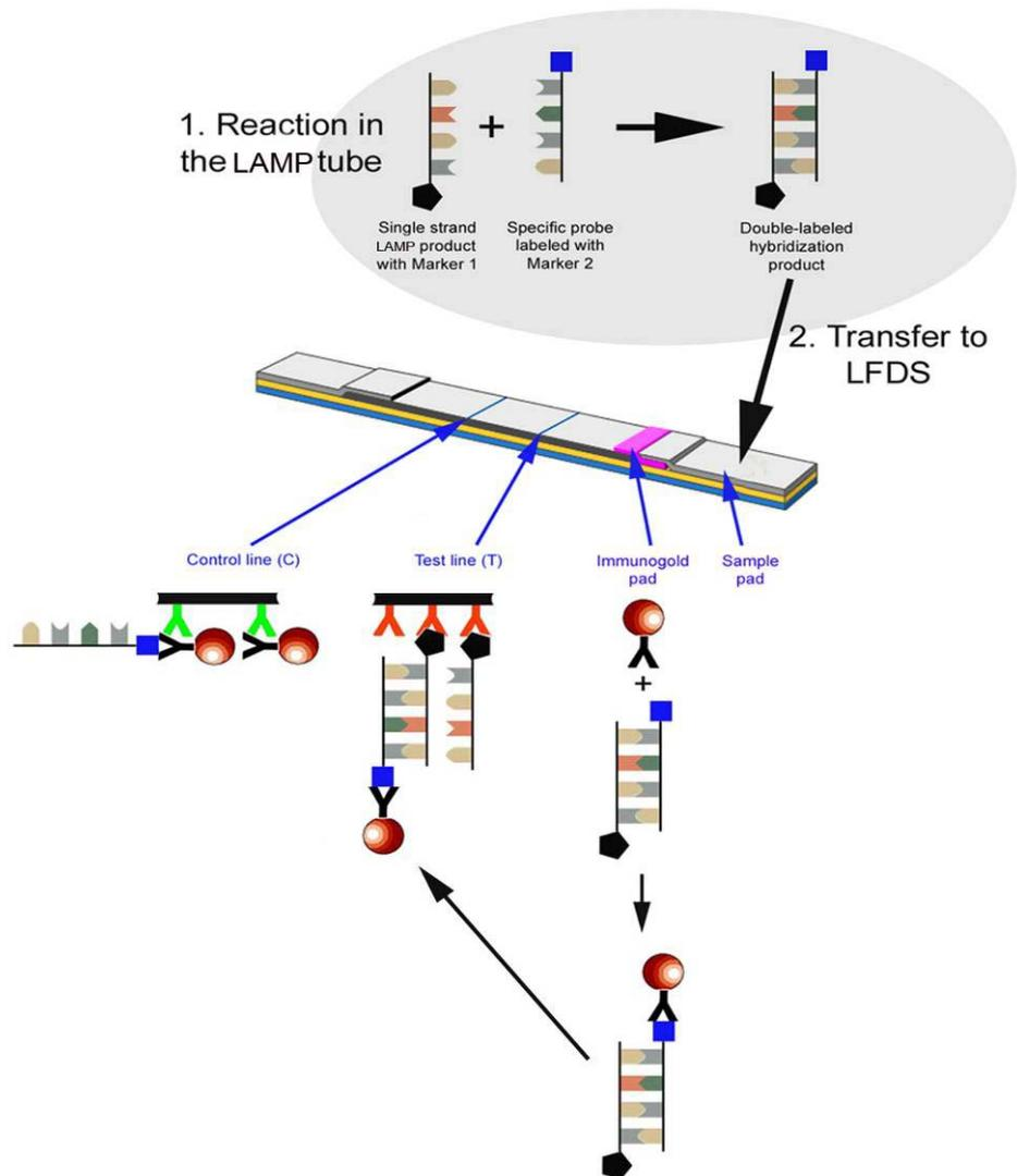
**Fig. 5.** Schematic diagram showing the mechanism of the lateral-flow dipstick (LFD).
