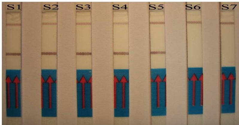
**Figure 17.** Photograph showing results of sensitivity tests using the lateral flow dipstick for detection of LAMP products from a plasmid template. Strip S1-6:  $10^5$  - 5 copies of recombinant plasmid in 100 ng of normal shrimp DNA, Strip S7: negative control (distilled water).
