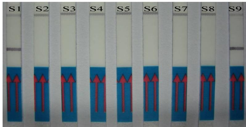
**Figure 19.** Photograph showing results of specificity tests using the lateral flow dipstick for detection of LAMP products using DNA of shrimp infected with various viruses. Strip S1-4: 100 ng of DNA extracted from HPV, MBV, WSSV and IHNV-infected shrimp, Strip S5-7 100 ng of DNA extracted from normal *P. monodon*, *M. rosenbergii* and *P. vannamei.*, Strip S8: negative control (distilled water), Strip S9: positive control.
