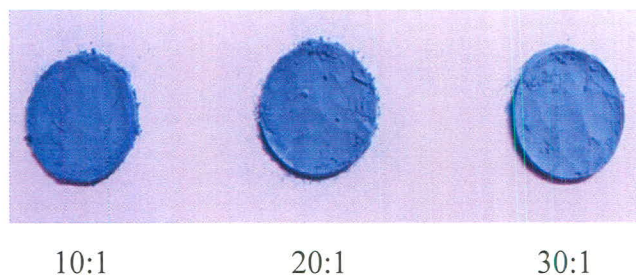
Figure 4.5 Bromothymol blue modified PCH at various weight ratio of clay and pH dye; 10:1, 20:1 and 30:1.
