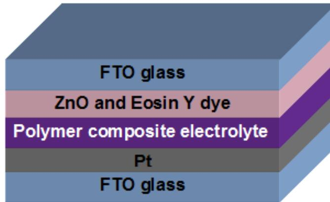
Figure 4.29 A schematic diagram of the DSSC.
