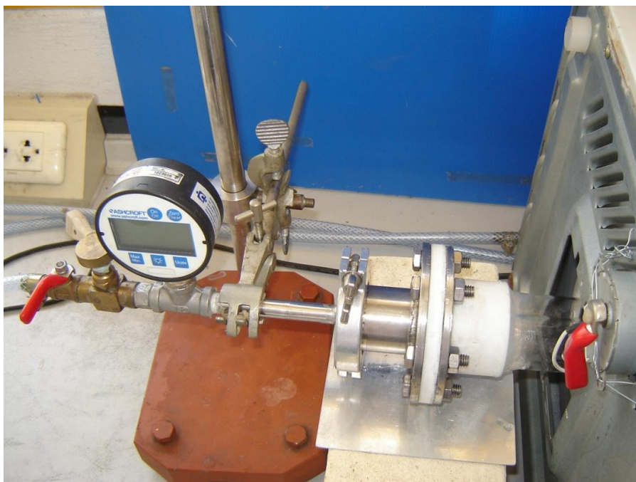
Figure 3.10 Pressure gauge of microwave plasma system.
