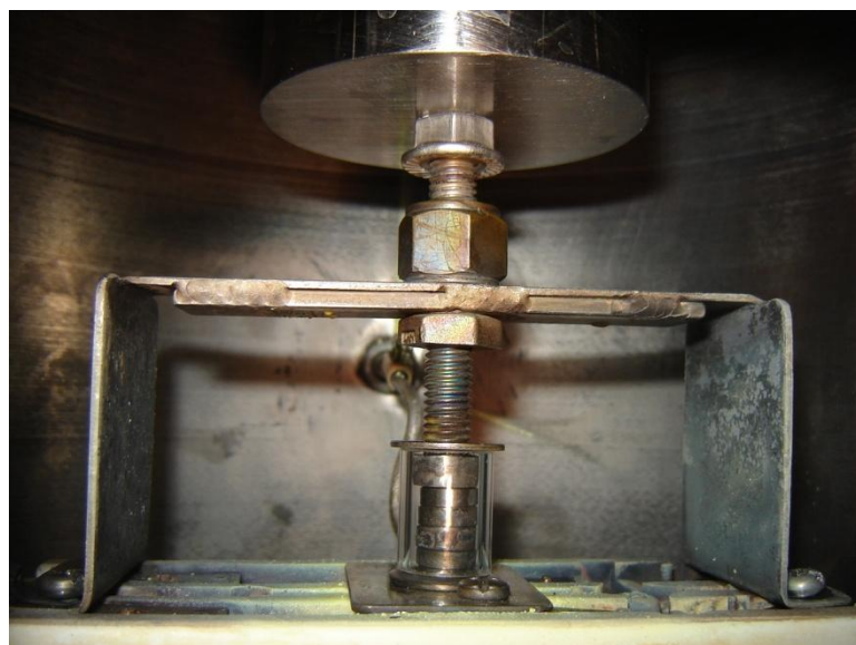
Figure 3.4 Photo of stainless steel electrodes contact with sample.
