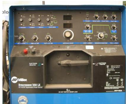
Figure 2.10 Welding power supply.
