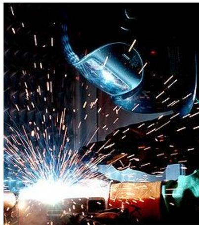
Figure 2.9 Gas metal arcs welding.
