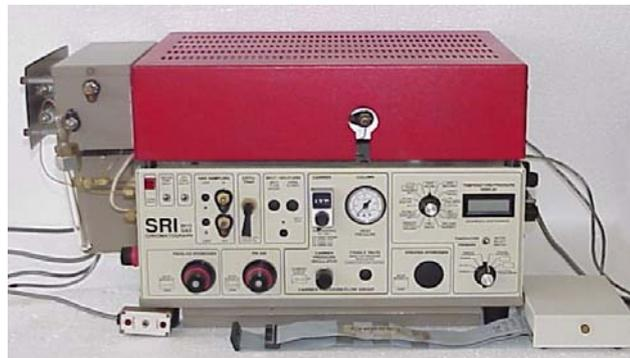
Figure 3.14 Gas Chromatography (GC) 8610C SRI Instrument, California.
