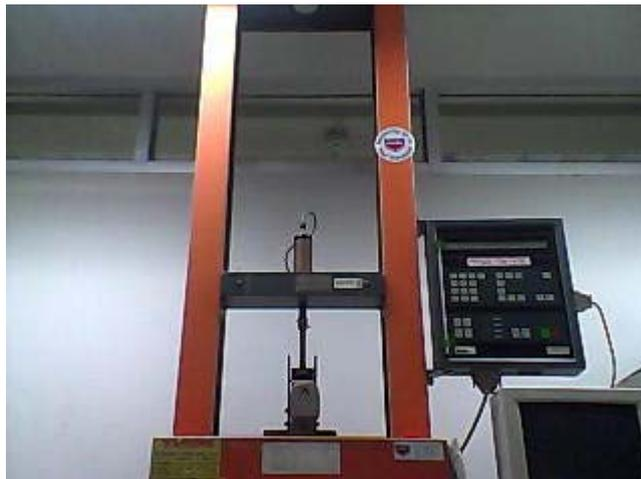
Figure 3.15. Universal Testing Machine (LR 100 N, LLOYD Instrument, United Kingdom).
