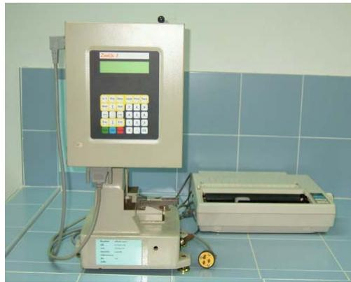
Figure 3.16 Pendulum Impact Tester (B5102.202 2 J, Swick I, Germany).
