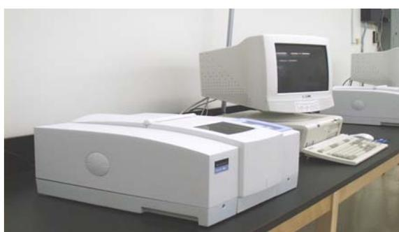
Figure 3.7 Fourier Transform Infrared Spectrophotometer (FTIR) Spectrum One, Perkin Elmer, California, United states.
