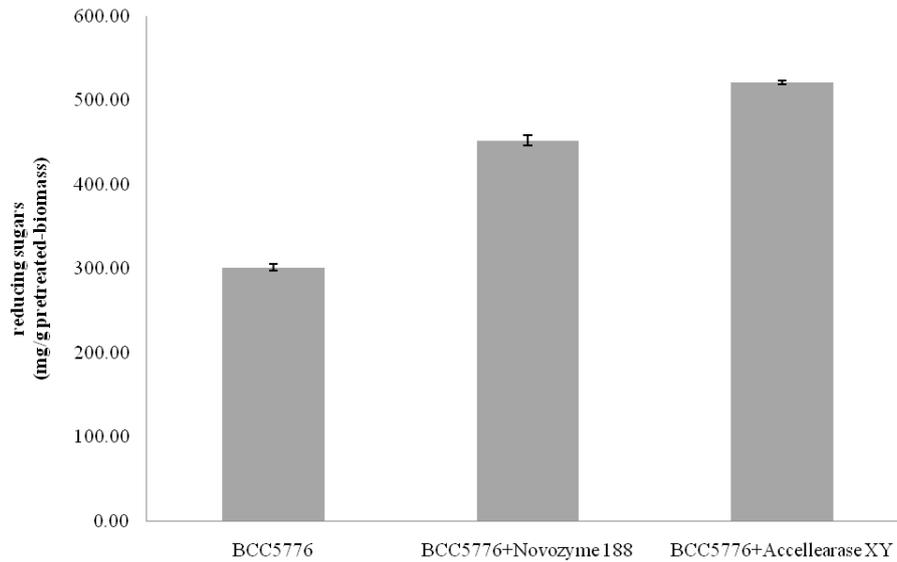
**Figure 4.15** The synergistic effects of Novozyme<sup>®</sup> 188 and Accellerase<sup>®</sup> XY on BCC5776 enzyme extract mixture on pretreated rice straw hydrolysis. The reactions contained 3 FPU/g of BCC5776 blend with the indicated amount of Novozyme<sup>®</sup> 188 (6.41  $\mu$ l) and Accellerase<sup>®</sup> XY (29.38  $\mu$ l). The reactions were incubated at 50 °C for 24 h.
