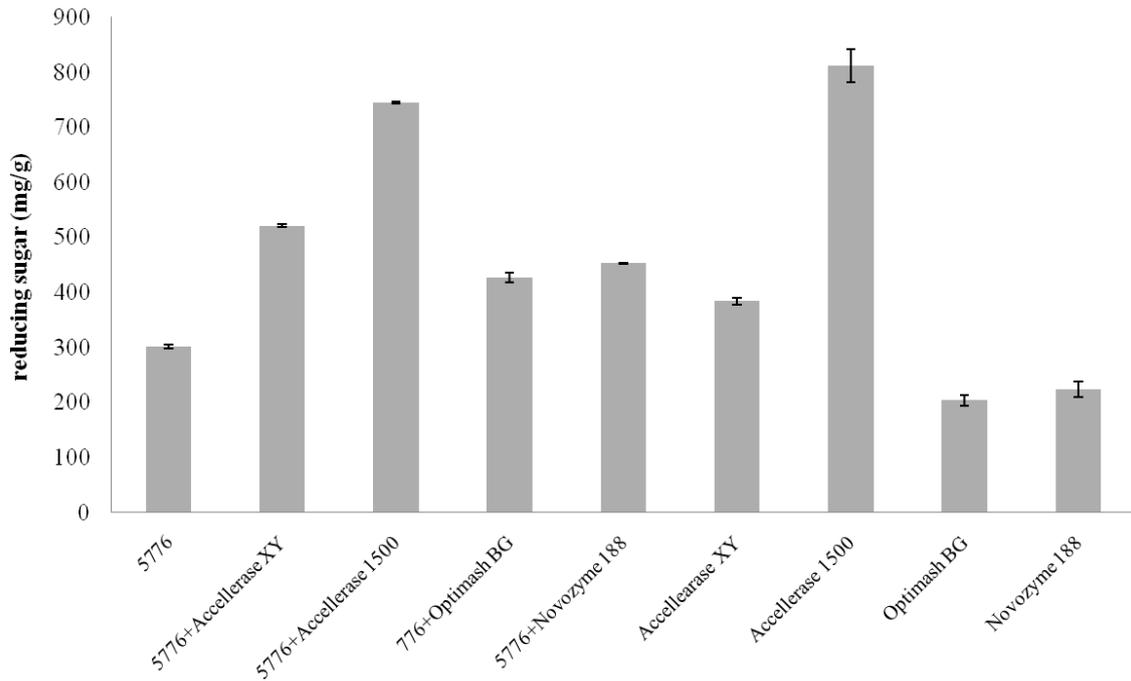
**Figure 4.14** The primary screen of different combinations of commercial enzymes and crude fungal BCC5776 enzyme extracts. A total of 0.29 mg protein of the BCC5776 enzyme extracts and 0.29 mg proteins of different commercial enzymes were mixed for a total enzyme dosage of different FPU/g loading of pretreated rice straw. The commercial enzymes control reaction contained 0.58 mg protein.
