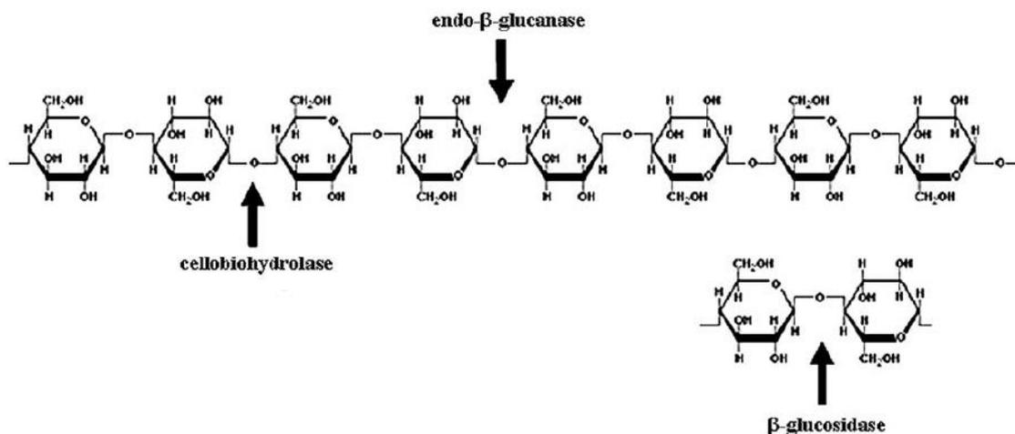
**Figure 2.4** Molecular structure of cellulose and site of action of endoglucanase, cellobiohydrolase and  $\beta$ -glucosidase [3].
