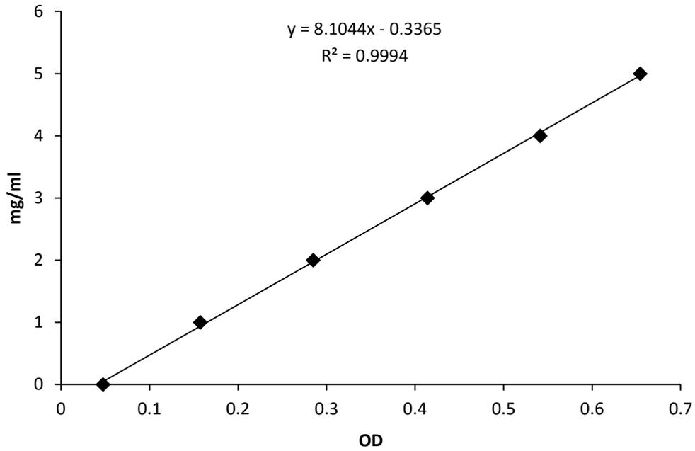
**Figure A.1.** Standard curve for analysis of the concentration of reducing sugar with DNS method (OD 560 nm)
