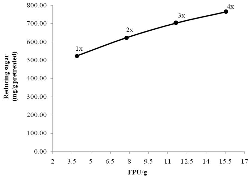
**Figure 4.18** The total reducing sugars versus FPU loading/g in pretreated rice straw hydrolysis. The reactions contained different FPU loading/g pretreated rice straw of a 44.4:20.6:35.0 (optimum ratio) BCC5776:Novozyme<sup>®</sup> 188:Accellerase<sup>®</sup> XY enzyme extract. The reactions were incubated at 50 °C for 48 h.
