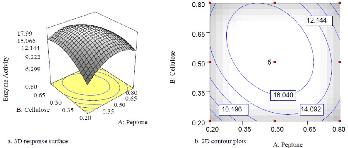
**Figure 1.6** Effects of peptone and cellulose concentrations (% w/v) on the production of cellulase [9].
