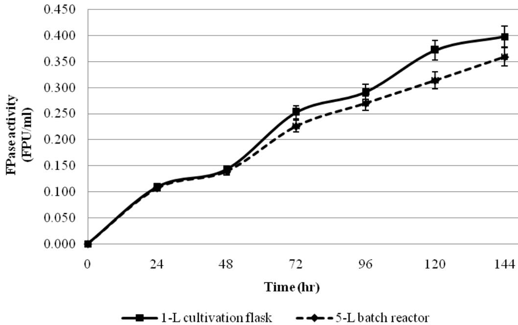
**Figure 4.5** Fermentation of the substrate scaled-up in 1-L cultivation flask and 5-L bioreactor performed under optimal conditions containing 2% (w/v) microcrystalline cellulose AVICEL<sup>®</sup>, 1% (w/v) OPEFB, 0.1% (v/v) lactose and 1% (w/v) soybean meal in distilled water, initial pH 5.8 and incubated at 30°C for 144 h with continuous shaking at 200 rpm.
