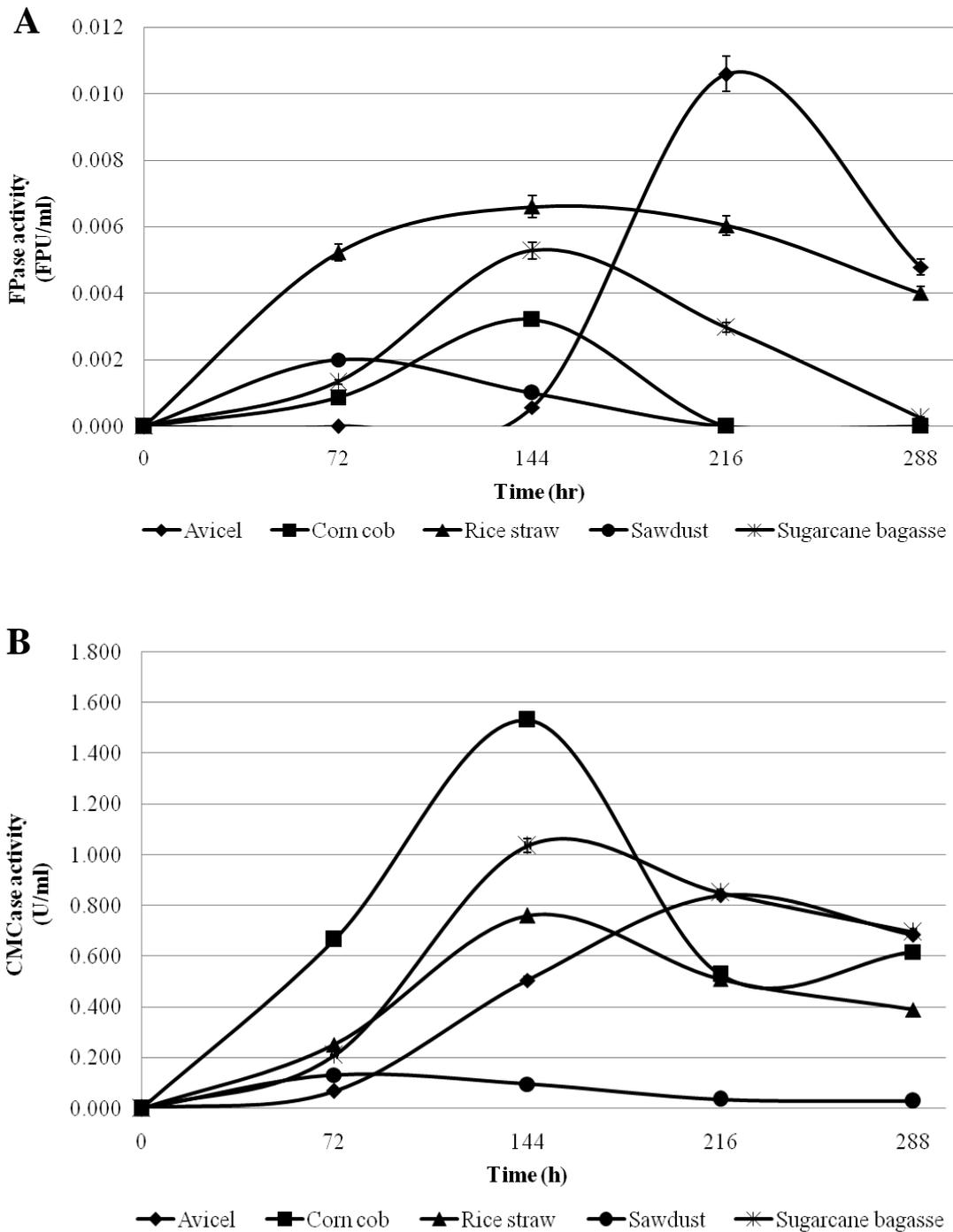
**Figure 4.1** Comparison of (A) filter paper cellulase (FPase) and (B) carboxymethyl cellulase (CMCase) activities from *C. globosum* BCC5776 during 288 h of fermentation. The working volume of 50 ml in 250 ml Erlenmeyer flask contained 4% (w/v) of different carbon sources (microcrystalline cellulose AVICEL<sup>®</sup>, corn cob, rice straw, sawdust and sugarcane bagasse) and 4% (w/v) of peptone in basal medium and incubated at 30 °C with continuous shaking at 200 rpm.
