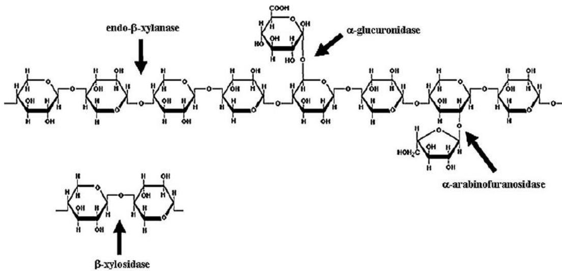
**Figure 2.5** Polymeric chemical structure of hemicellulose and targets of hydrolytic enzymes involved in hemicellulosic polymer degradation [3].
