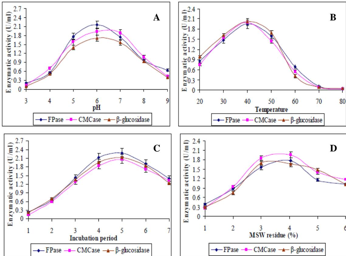
**Figure 1.7** Effect of cellulase production (U/ml) by *Trichoderma viride*: (A) pH, (B) temperature, (C) incubation time, (D) concentration of MSW used as alternative carbon source [10].
