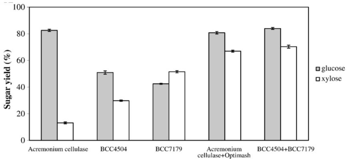
**Figure 1.14** Effect of enzyme mixtures hydrolysis of 5% (w/v) pretreated bagasse in 50 mM sodium acetate buffer, pH 5.0, for 72 h at 45 °C. Enzymes used included 5FPU/g substrate of *Acremonium* cellulase, 20 U (as xylanase activity)/g substrate of Optimash BG, 5 FPU/g substrate of cellulase preparation from *P. chrysogenum* BCC4504, and 10 U (as  $\beta$ -glucosidase activity)/g substrate of enzyme preparation from *A. flavus* BCC7179 [16].
