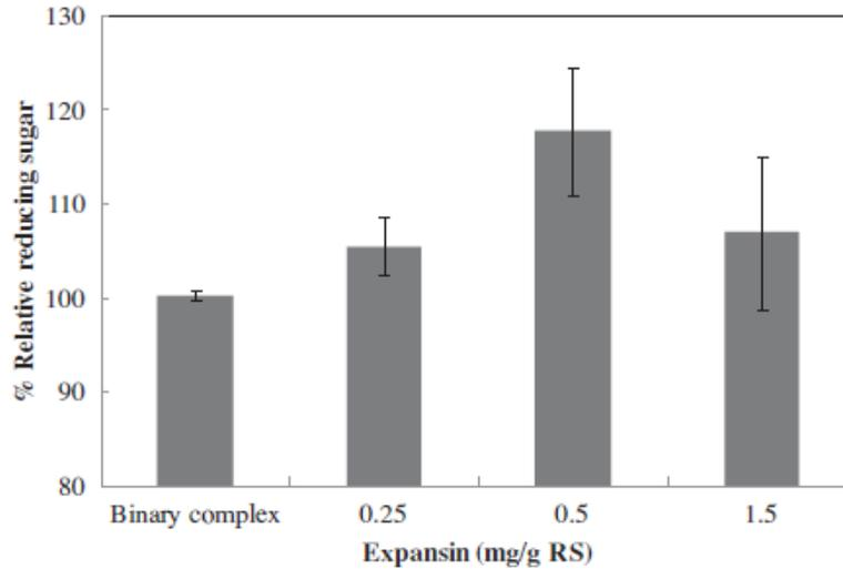
**Figure 1.17** The synergistic effect of expansin on the binary Celluclast™-BCC 199 enzyme extract mixture on rice straw hydrolysis. The reactions contained 5 FPU/g of a 50:50 Celluclast™:BCC enzyme extract blend with the indicated amount of expansin. The reactions were incubated at 50°C for 48 h [19].
