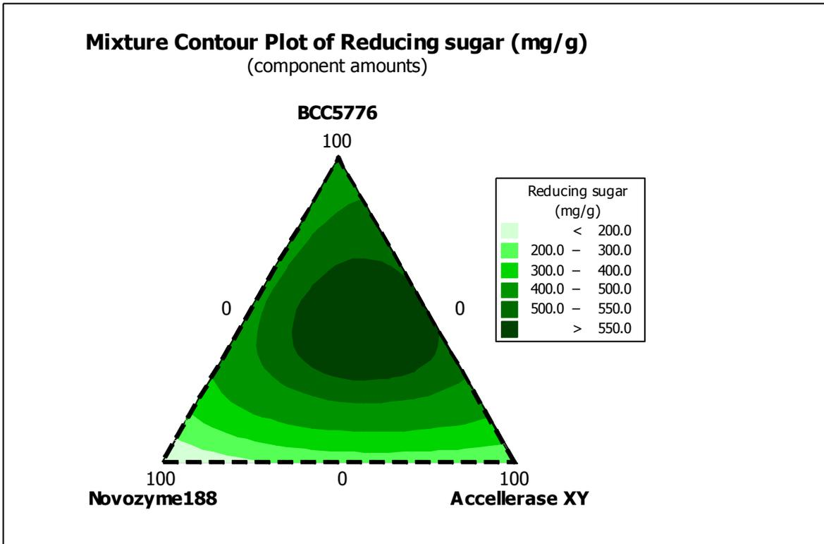
**Figure 4.17** The ternary plots of the experimental design optimization of the ternary enzyme complex. The contour plot represented the different levels of reducing sugar. 100% component amount always equals to 400  $\mu$ l.
