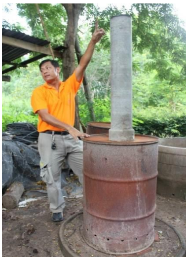
Figure 4.19 Kiln used in biochar production at Huay Sai Royal Development Study Center, Phetchaburi Province
