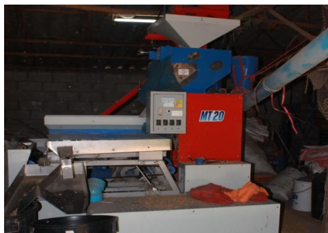
Figure 4.10 Rice grinding machine at the granary, Mae Taeng District, Chiangmai Province
