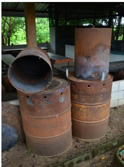
Figure 4.11 Kiln used in biochar production at Mae Taeng District, Chiangmai Province
