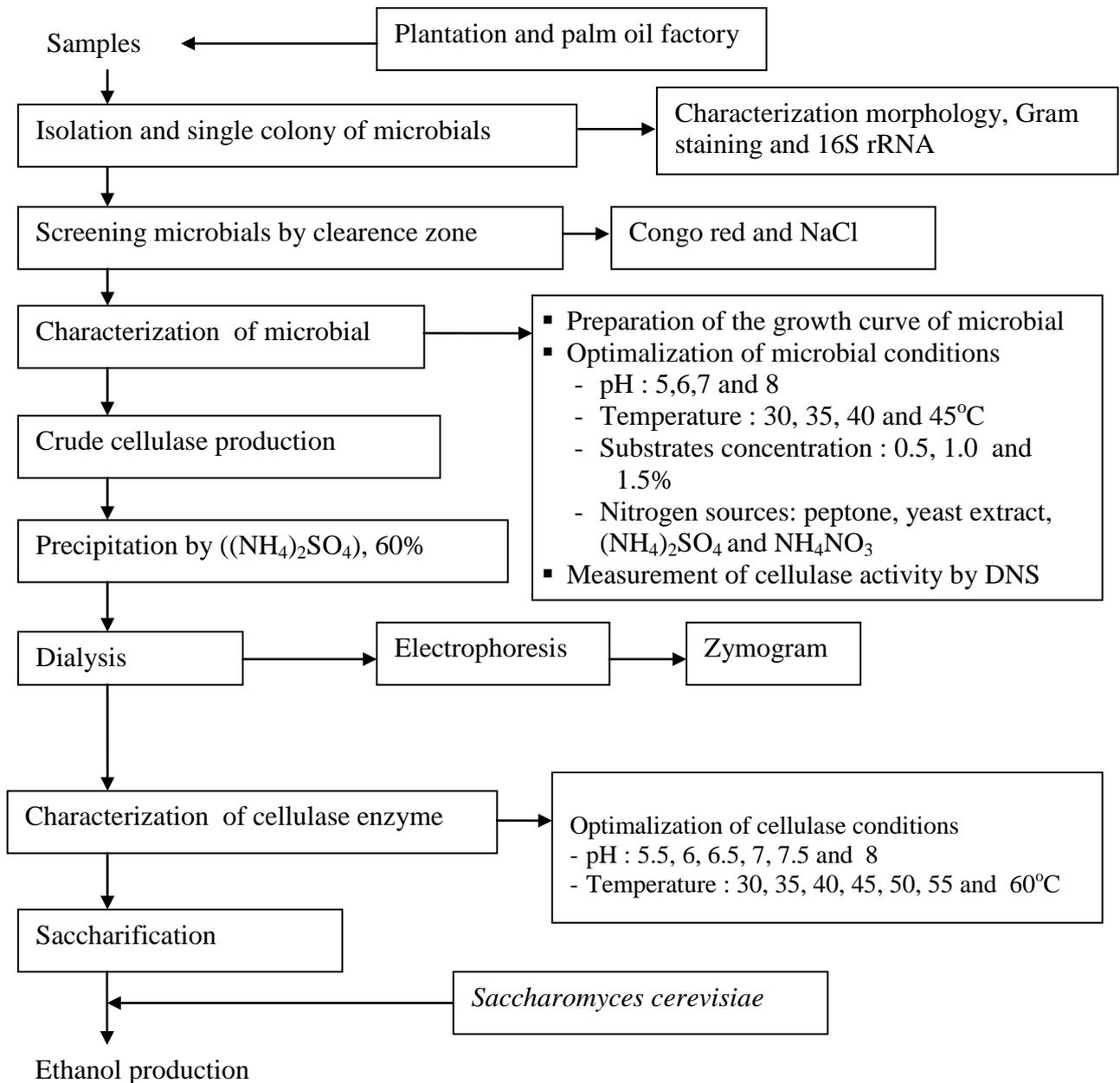
**Figure 3.2** Flow chart of the ethanol production from microbial cellulase associated with the palm oil industry.
