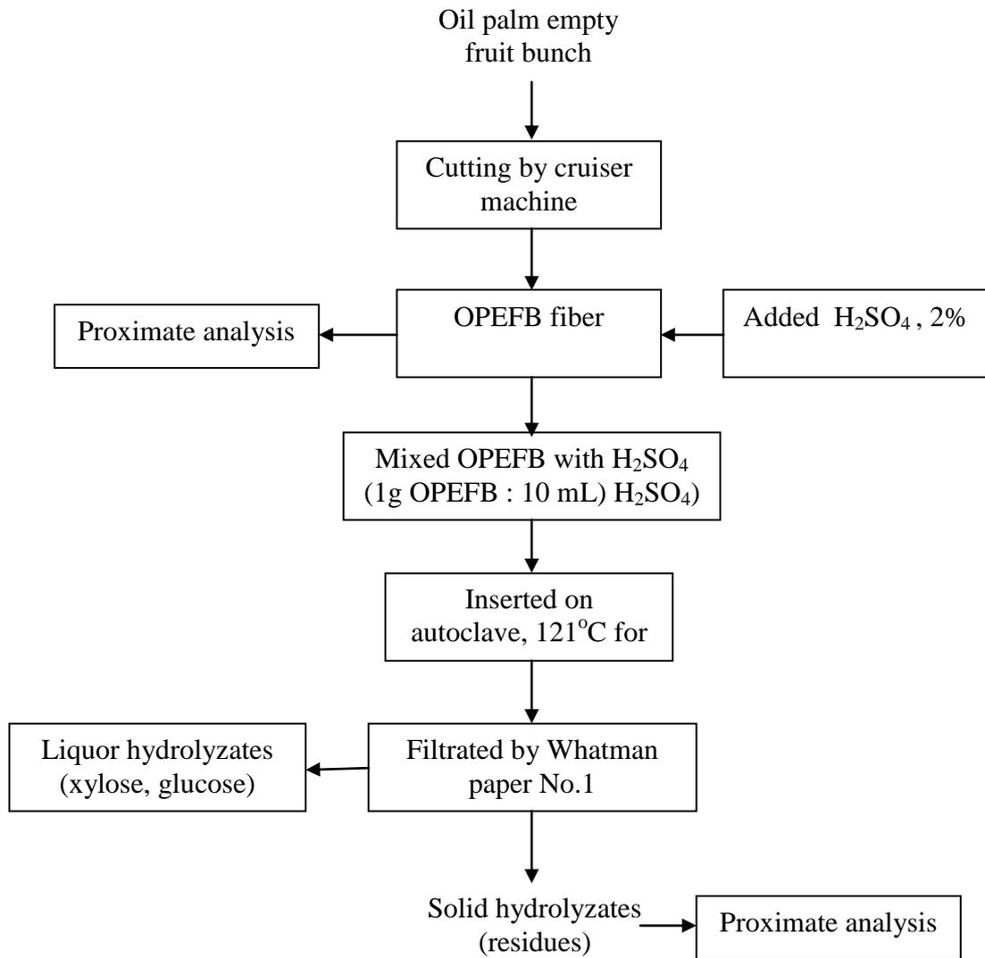
**Figure 3.1** Flow chart preparation of residue from acid hydrolysis of OPEFB
