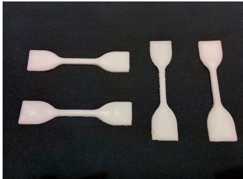
Figure 4.4 ASTM D638 Type IV specimens of PBS-EVA blends
