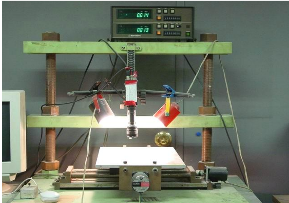
Figure 2.26 Machine to digitise the coordinates of markers on taken photo placed on movable table equipped with high accuracy servo motor (Kongkitkul, 2004)
