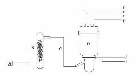
Figure 3.1 Schematic diagrams of the pervaporation apparatus
