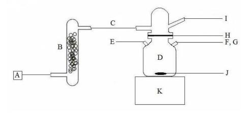
Figure 3.2 Schematic diagrams of the vapor permeation apparatus
