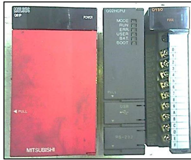
Figure 3.4 Power supply model Q61P CPU unit model Q02HCPU Output module model QY50
