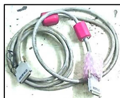
Figure 3.3 Cable GT15-QC30B link between PLC and Touchscreen
