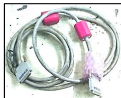
Figure 3.3 Cable GT15-QC30B link between PLC and Touchscreen
