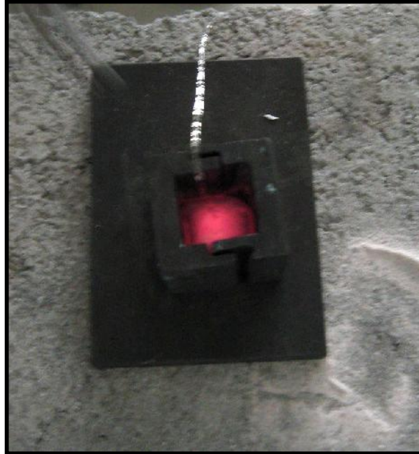
Figure 3.7 Glasses in stainless steel mould.
