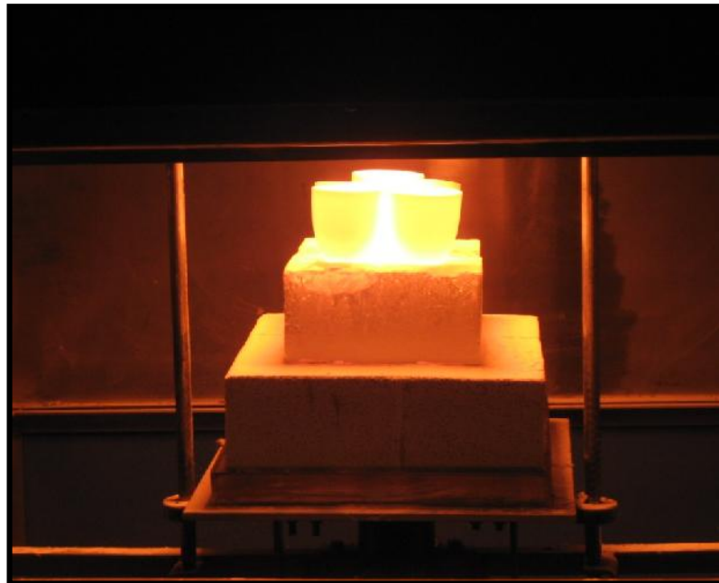
Figure 3.4 Melting at 1,100 °C.
