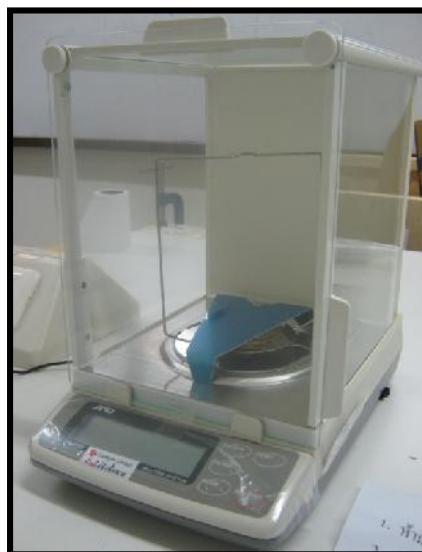
Figure 3.13 The sensitive microbalance for density determination.
