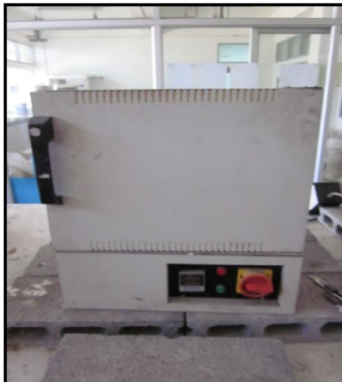
Figure 3.8 High temperature electrical furnaces for glass annealing.
