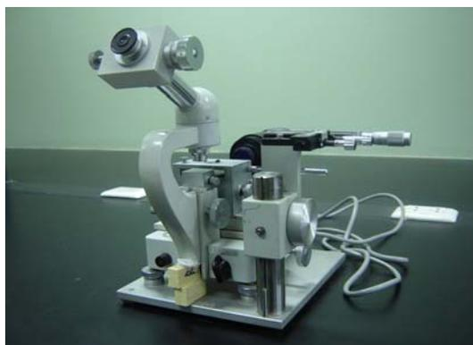
**Figure 4.5** Contact angle goniometer.
